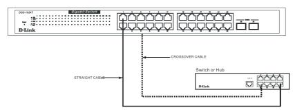
Figure 2- 5. Switch connected to a port on a hub or switch using either a straight or crossover cableany standard Ethernet cable is fine
